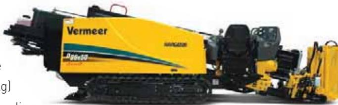
(6681 Nm) of rotary torque and 33,000 lb (14,969 kg) of thrust with 36,000 lb (16,329 kg) of pullback.
