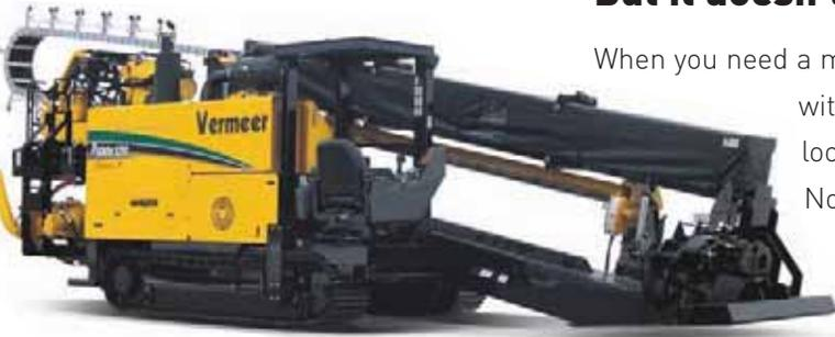
Being the only system of its kind in the UK the D100/120 offers power and efficiency at its best. Powered by a John Deere 6068 engine, the D100x120 Series II features 12,000 ft-lb (16,270 Nm) of rotational torque and 100,000 lb (45,359 kg) of pullback. This commanding combination results in ease and efficient installation of larger diameter pipes. George Aitkenhead, AMS Group Managing Director said;
